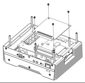
Step 6: Close the bottom case of AEC-6625 and fasten the six screws
