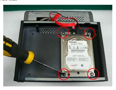
Step 4: Close the bottom cover of the AEC-6625 and fasten the screw
