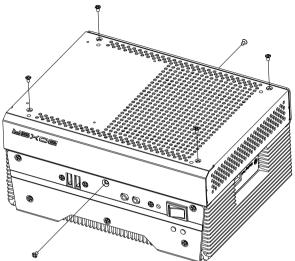
Step 7: Fasten the four screws to install the two bracket
