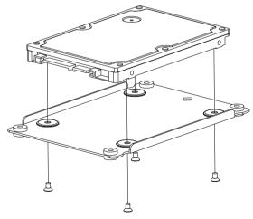
Step 4: Fasten the four screws to fix the HDD bracket with the bottom case of AEC-6625
