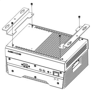
Step 2: Unfasten the six screws to release the bottom case of the AEC-6625
