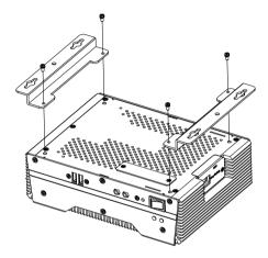
Step 2: Unfasten the five screws to release the bottom cover of the AEC-6625
