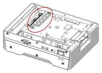
Step 3: Adhere the heat spreading pad to the RAM
