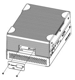
Step 2: Insert the CompactFlash™ and finish the installation
